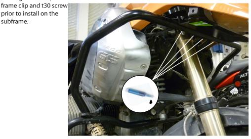
Rest the upper crash bar onto the existing lower crash bar assembly. Use a few drops of threadlockerand and start the (4) M6 x 35 socket head cap fasteners with (4) M6 washers into the upper bracket. All bar fasteners should be left loose.
