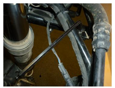
(3) Turn the handle bars to access the M6 screws with allen key. Use the M10 socket tool under the bracket to tighten the (2) M6 nylock nuts. Now tighten the (2) OEM T25 beak screws.
