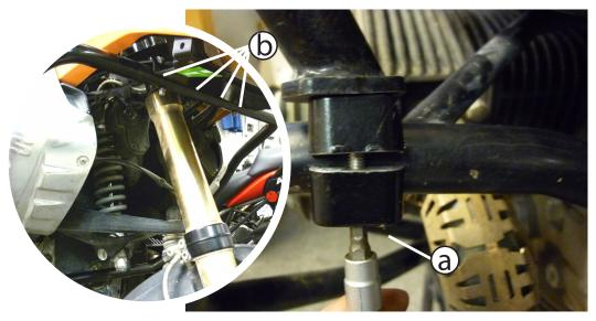
a) Now slowly tighten both sets of clamps, alternating between front and rear screws so the clamps compress evenly.
